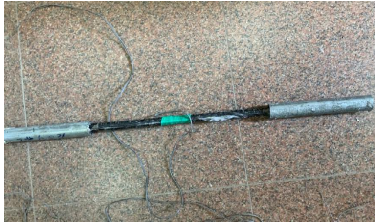
Figure 5. Overall View of Failed HFRP Specimen core
