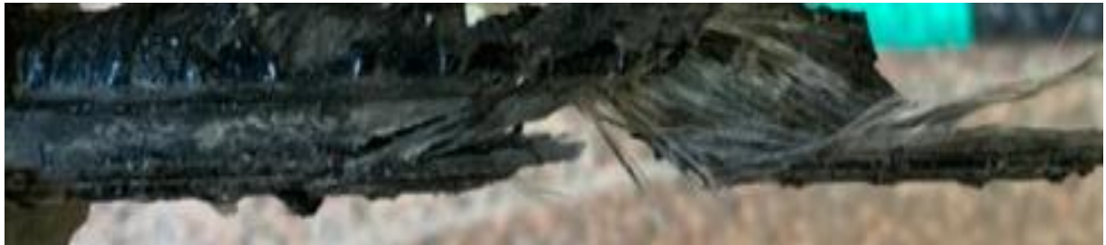
Figure 5. Overall View of Failed HFRP Specimen core
