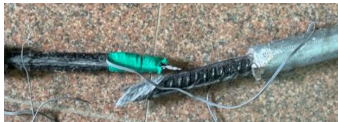
(c) HFRP bar with steel rebar in core at failure
