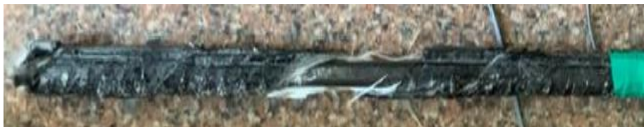
(a) Normal FRP failure
