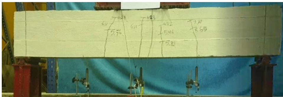
Figure 24. Ductile flexural failure mode of hybrid beam B-7-H.
