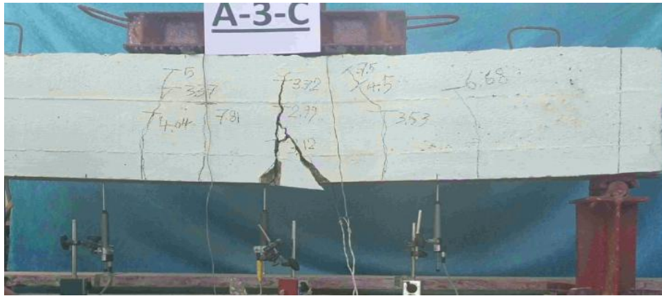
Figure 14. Flexure failure at mid span of beam A-3-C.
