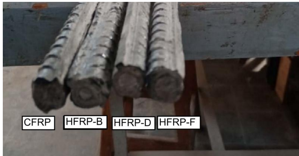
Figure 3. : Final product for development of FRP Hybrid Bars.
