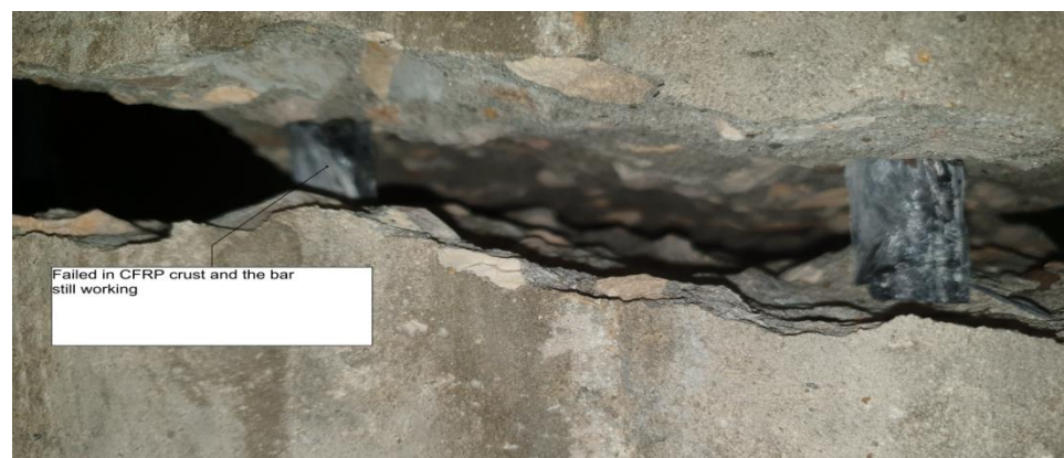
Figure 22. For type (B,D, and F)"carbon type," the impact of hybridization in overcoming the rapid rupture.
